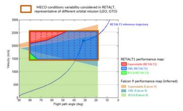
Figure 7 Feasibility map for the recovery of RETALT1 (and comparison with reconstructed Falcon 9 performance [8])
