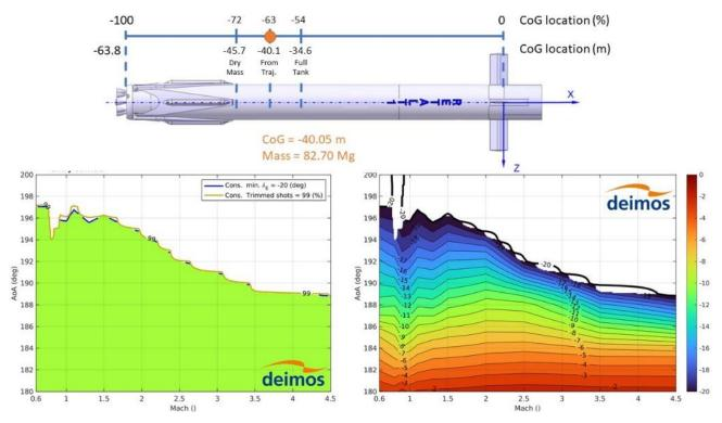
Figure 8 Dispersed (Monte Carlo) AoA entry corridor for the reference propellant loading, planar fins configuration, aerodynamic phase
