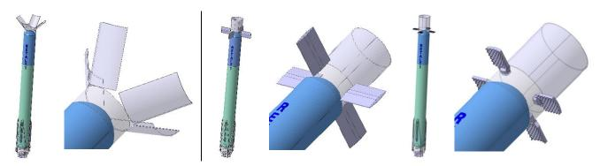
Figure 3 RETALT1 ACS configurations: interstage petals (left), planar fins (center), and grid fins (right) [3]
