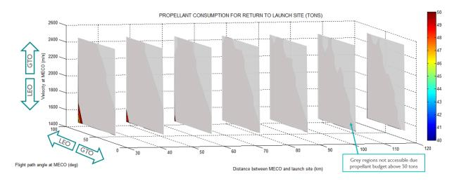
Figure 6 End-2-end propellant budget as function of conditions at MECO, RETALT1 PF configuration, RTLS
