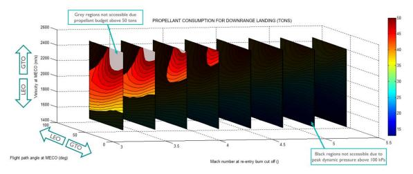
Figure 5 End-2-end propellant budget as function of conditions at MECO, RETALT1 PF configuration, DRL
