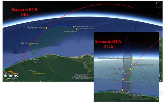
Figure 10. Google Earth representation of the consolidated return trajectories: RTLS (R1 A) and DRL (R1-B) scenarios.
