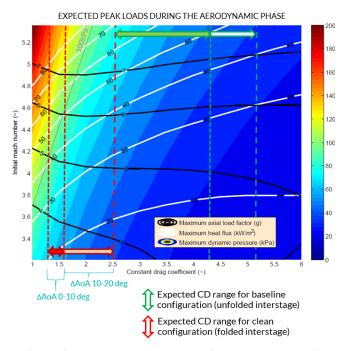
Figure 4 Expected peak loads during the aerodynamic entry, RETALT1 aerodynamic phase
