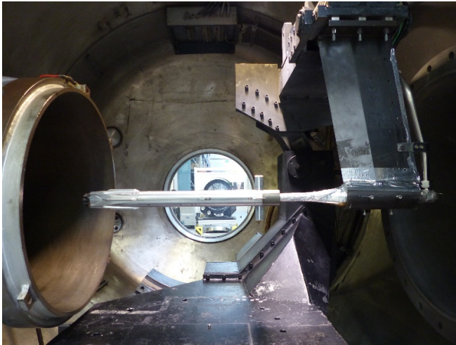
Fig. 2. The RETALT1 model in the H2K facility.
