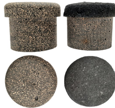
Fig. 16: Novel cork TPS material (TPS05) before (left) and after (right) test in L2K at DLR. Top: profile view, Below: surface view.
