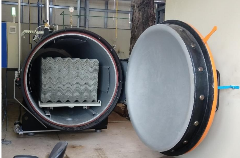
Figure 1 - The autoclave Fhaizer used as a chamber for accelerated carbonation, model FZR INDL/885-2017, Brazil. The diameter is 1.6 m, and the internal volume is 7.8 m 3 . 200 sheets were placed inside and prepared for the beginning of the accelerated carbonation process.
