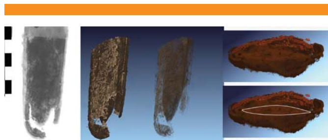
Figure 5: \mu -CT scan image of the sword within its scabbard and section (Lent, BAMN (Bureau Archeologie & Monumenten, gemeente/ Nijmegen)) - 220 kV, 85 W, 1000 ms, voxel size: 180 \mu m.
