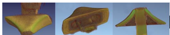
Figure 4: \mu -CT scan image of the internal structure of the copper alloy pommel of a sword from the Merovingian burial site of Lent (Nijmegen, Netherlands) BAMN (Bureau Archeologie & Monumenten, gemeente/ Nijmegen). 50 W-1000 ms - voxel size: 50 \mu m.
