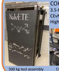
COH-NaI-2 (NaIvETe) 3.5-t scintillation detector CEvNS search and CC High/low gain digitization
