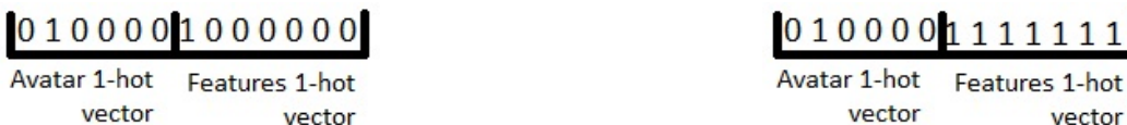
(a) The representation of the vector in the training phase. (b) The representation of the vector in the testing phase.
