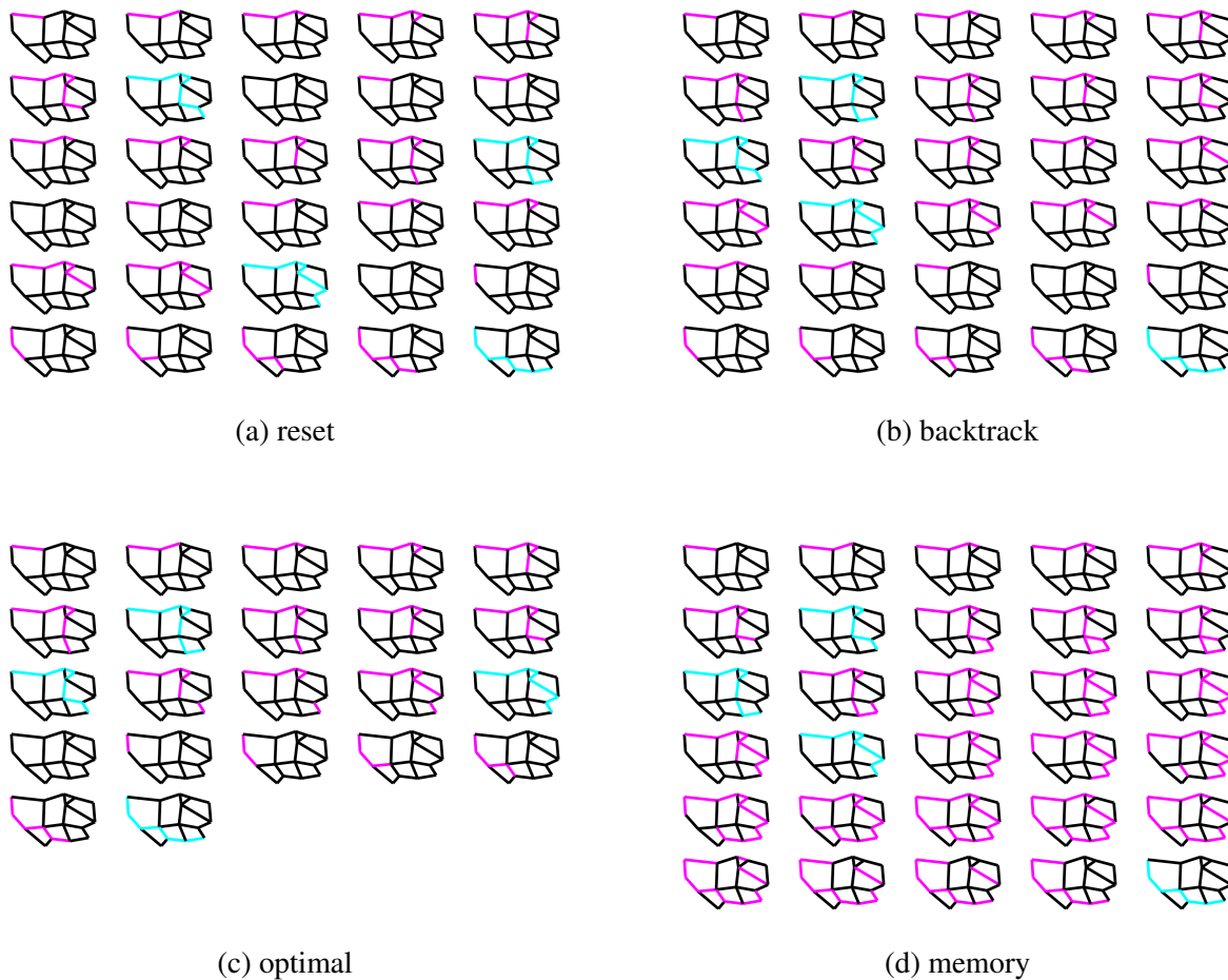
Figure 2: Visualization of different methods of switching between paths. Action sequences are displayed row-wise. Cyan color: complete path, magenta color: incomplete path.
