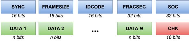
Fig. 2. Message format of a C37.118 frame, where most significant byte (first byte of SYNC) is transmitted first
