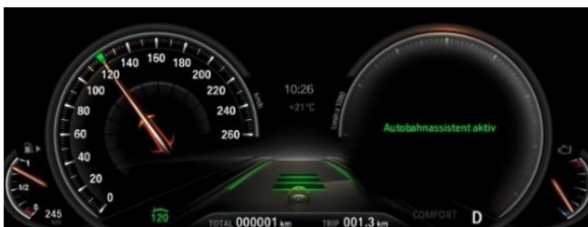
Figure 1: Mode information shown on instrument cluster with a verbal indicator "Automation assistant is active" [32].
