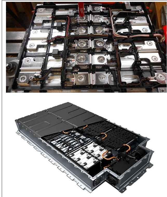
Figure 37: BMW i3 laser welded cell connections 48 and battery pack
