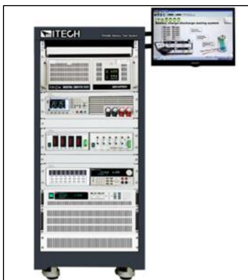
Figure 46: A bi-directional power supply and separate data acquisition units assembled in a mobile arrangement 52
