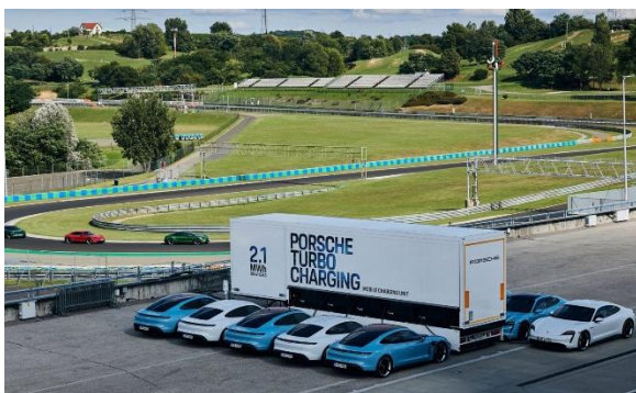
Figure 57: Mobile fast charging station from Porsche for track days
