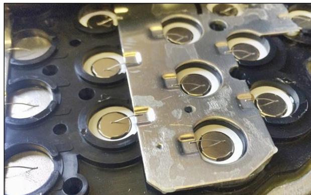
Figure 35: Ultrasonically Welded Wires on Cylindrical Cells 45
