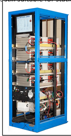
Figure 53: Nuvation storage system with Nissan Leaf modules
