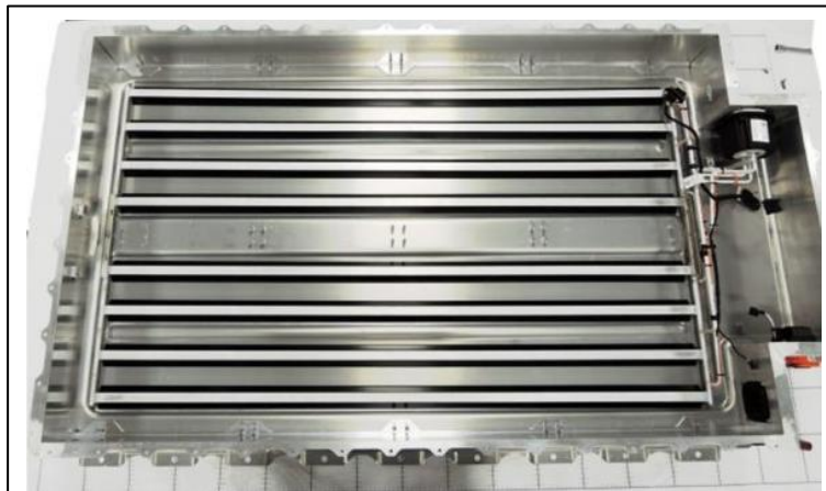
Figure 40: Evaporator/cooling plate at the bottom of a BMW i3 battery pack (public source)
