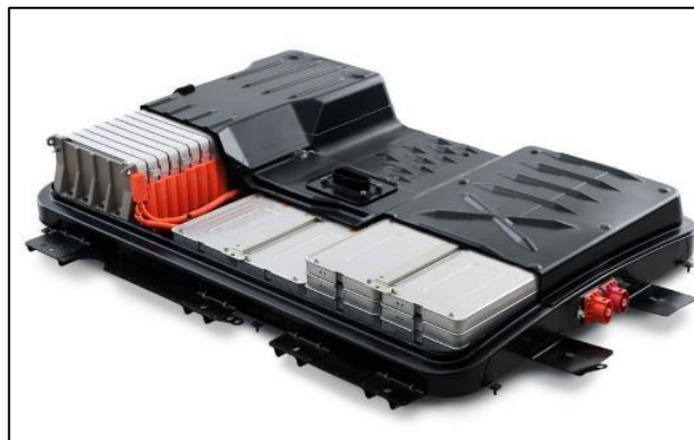
Figure 42: Nissan Leaf . passive air-cooled battery pack (public source)
