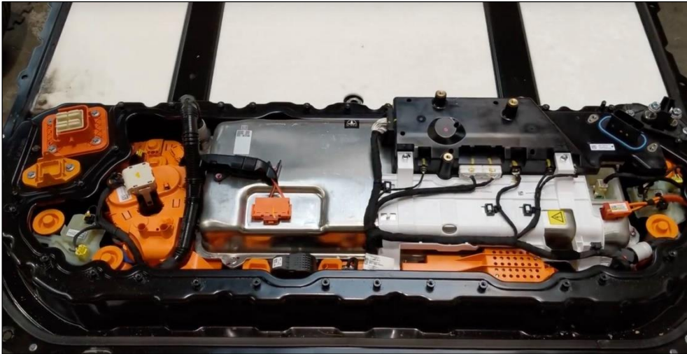
Figure 21: Tesla Model 3 battery pack with extensive integration: e.g. HV interconnections, DC/DC converter and fast charging port. 31
