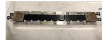
Fig. 2: Photo of the assembled cooling structure with micro-pipes and interconnection blocks on the two sides.
