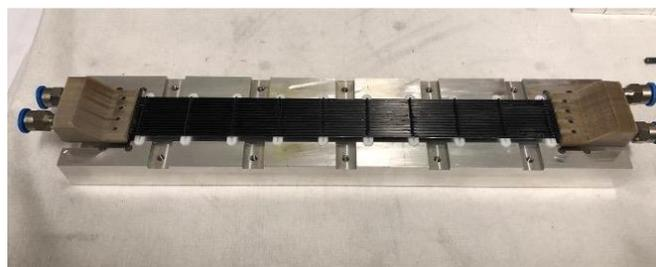
Fig. 2: Photo of the assembled cooling structure with micro-pipes and interconnection blocks on the two sides.
