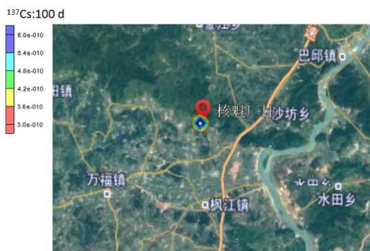
Fig. 4.18. Concentration and groundwater pollution range of ^{137}\text{Cs} after pollutant leaking for 100 days
