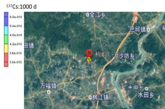
Fig. 4.19. Concentration and groundwater pollution range of ^{137}\text{Cs} after pollutant leaking for 1,000 days
