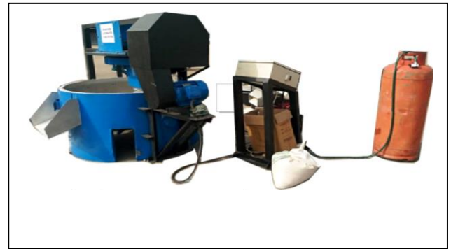
Fig. 1: Gas fired and automated garification machine
