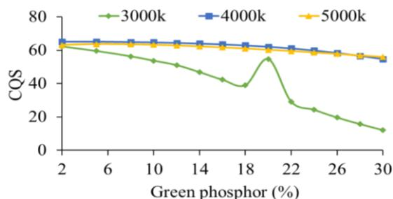
Figure 9.  $\text{Sr}_3\text{WO}_6:\text{U}$  concentration functions as the color quality scale of WLEDs
