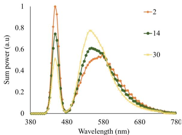
Figure 4.  $\text{Sr}_3\text{WO}_6:\text{U}$  concentration functions as the emission spectra of 4000 K WLEDs
