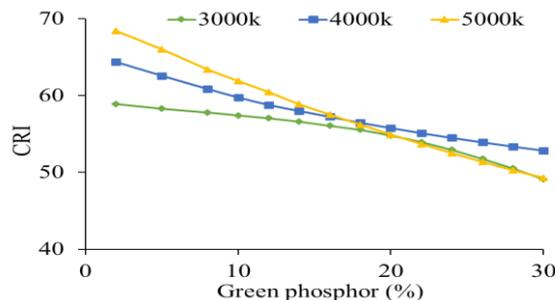
Figure 8.  $\text{Sr}_3\text{WO}_6:\text{U}$  concentration functions as the color rendering index of WLEDs
