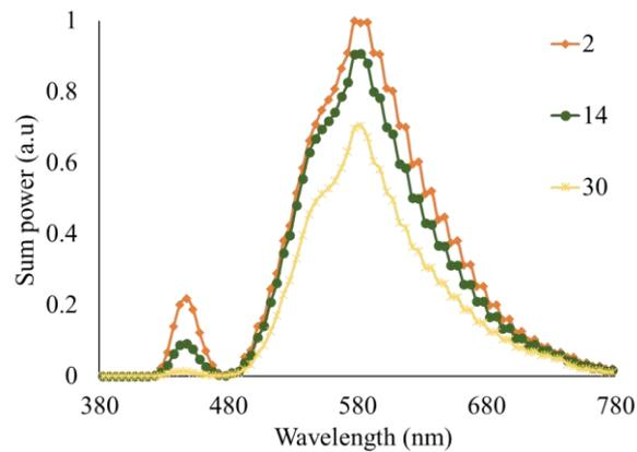
Figure 3.  $\text{Sr}_3\text{WO}_6:\text{U}$  concentration functions as the emission spectra of 3000 K WLEDs
