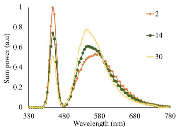
Figure 5.  $\text{Sr}_3\text{WO}_6:\text{U}$  concentration functions as the emission spectra of 5000 K WLEDs
