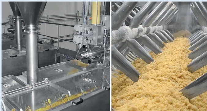
Figure 8.b [Process step 5] Example of dough mixer. Images courtesy of Italtast srl of Fidenza, Italy.
