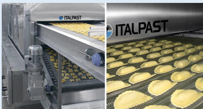
Figure 8.c [Process step 8]: A conveyor belt carries the pre-dried ravioli to a pasteurizer, which uses overheated steam with two drying tiers so that the raviolis are ready for cooling and packaging. Hot air and steam are not recycled to avoid potential cross contact. Images courtesy of Italtast srl of Fidenza, Italy.
