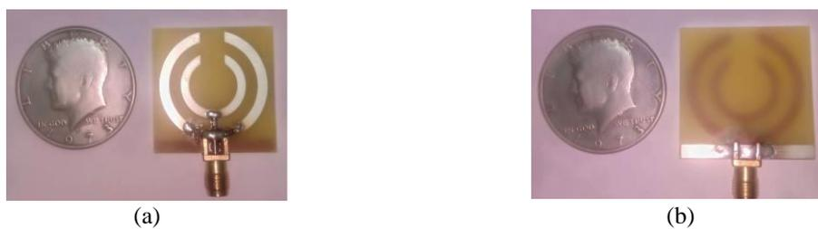
Figure 5. The fabricated compound reconfigurable antenna (a) radiation plane and (b) ground plane
