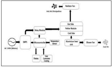
Fig. 3: Block Diagram of the System.
