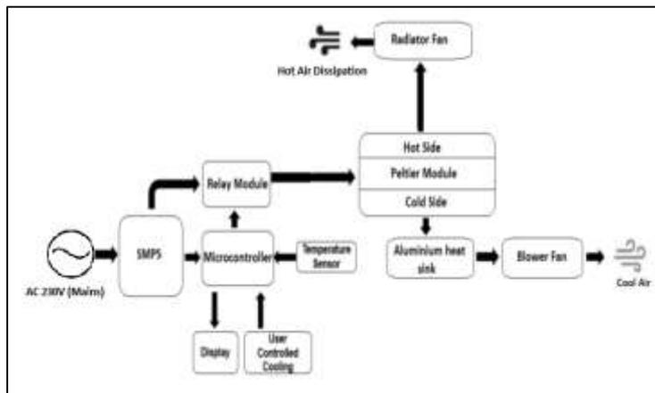
*Fig. 3: Block Diagram of the System.*
