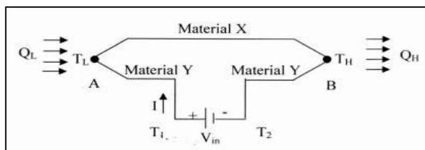
**Fig. 2:** Circuit to illustrate Peltier Effect [12].
