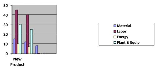
This chart illustrates conservation of value in a product that is remanufactured versus one that is recycled. The relative costs of material, labour, energy and the contribution of plant and equipment to a product in its manufacture are shown on the left. Remanufacturing preserves much of this value while adding a second life to the product. In contrast, recycling shreds the product in an attempt to
