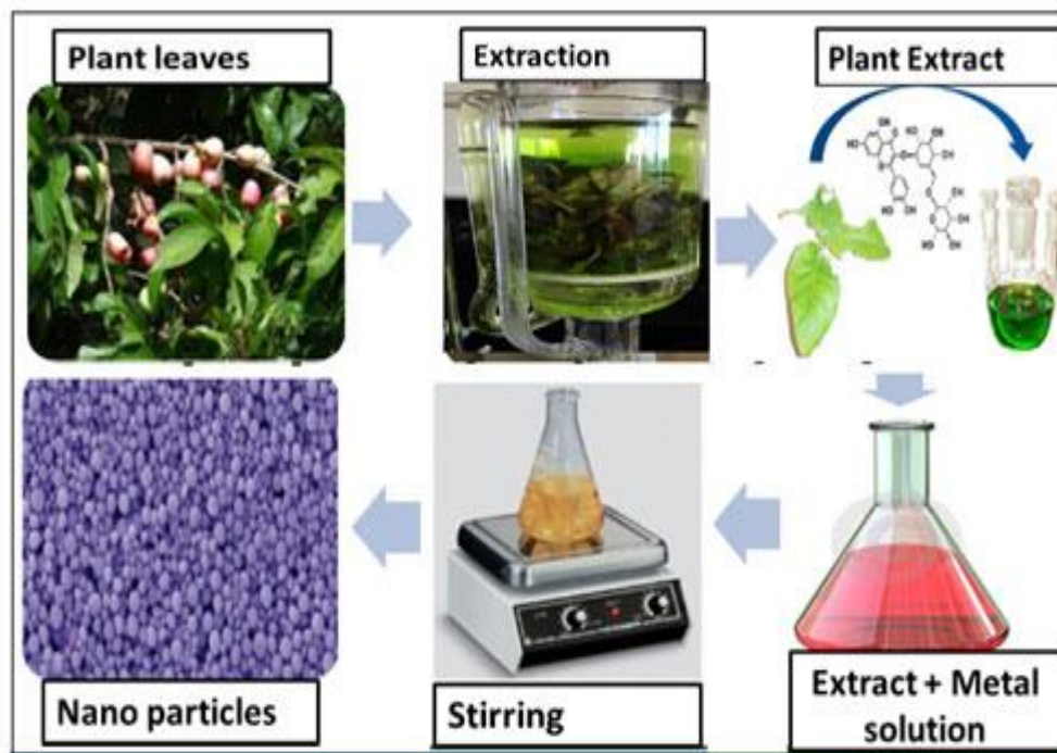
Figure 1: A schematic diagram of green synthesis of metal
