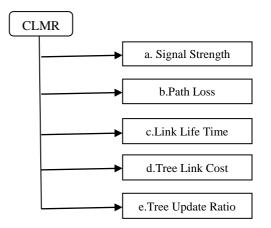
a) Signal strength: If a non-member node wants to join the group, then it should have a better quality of signal strength which can be derived as:  $S_s = (S_t *G)/dn * Pl$  Where  $S_s : Signal Strength St : Packet transmitted with t$
