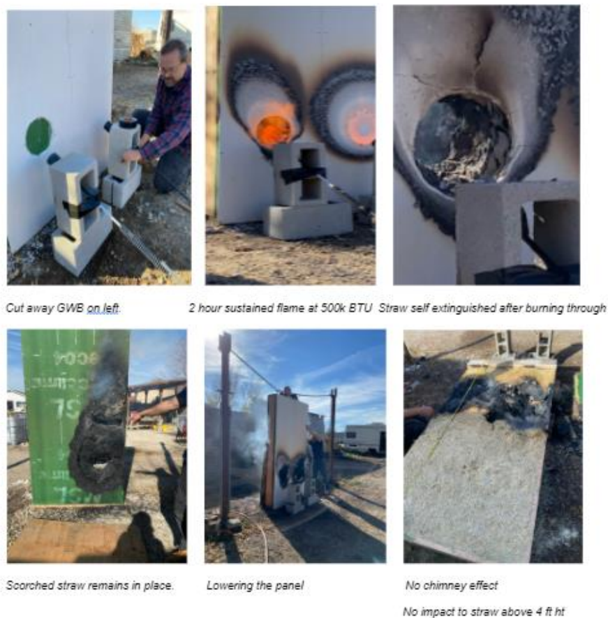
Figure 8: Informal fire test on Strawtegi prototype panel
