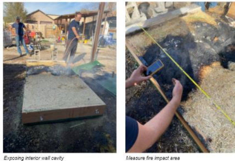
Figure 9: Informal fire test demonstrating limited flame spread inside the panel
