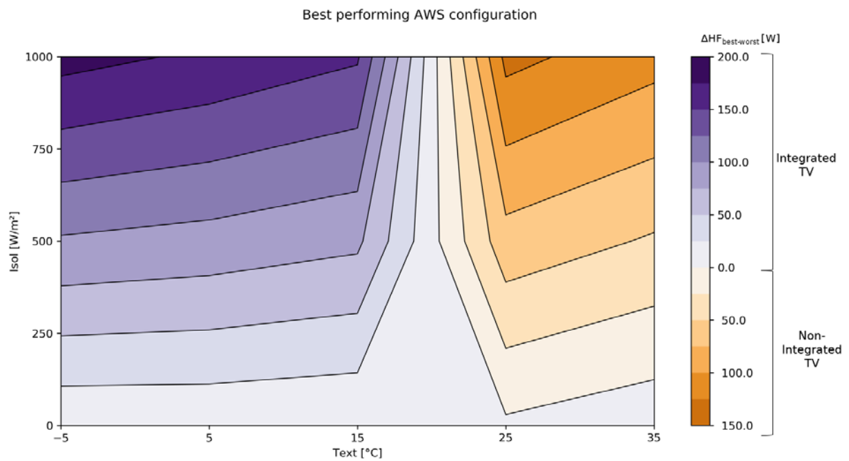
Figure 15. Best performing AWS configuration: integrated vs non-integrated TV (purple colors: AWS with integrated TV performs better, orange colors: AWS with non-integrated TV performs better)
