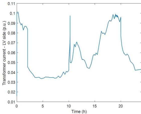
Fig. 7. Current profile on the secondary side of the OLTC transformer.
