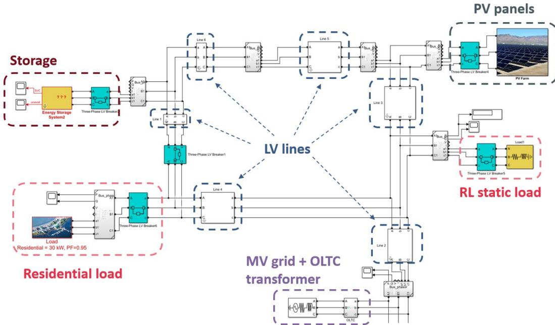
Fig. 2. Simulink diagram of the benchmark model (phasor version).
