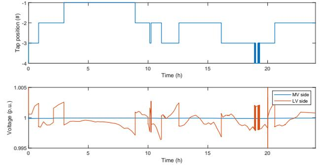
Fig. 6. Tap position (top) and voltage on primary/secondary side (bottom) of the OLTC transformer.
