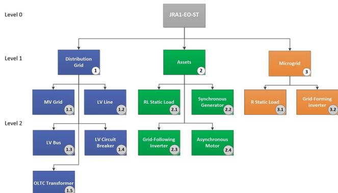
Fig. 3. System breakdown of the benchmark model (dynamic version).
