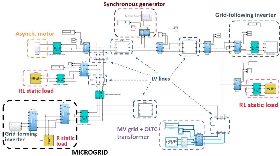
Fig. 1. Simulink diagram of the benchmark model (dynamic version).
