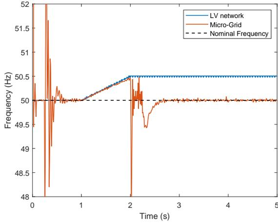
Fig. 4. Frequency profile in the LV network (blue) and estimated frequency in the microgrid (red).
