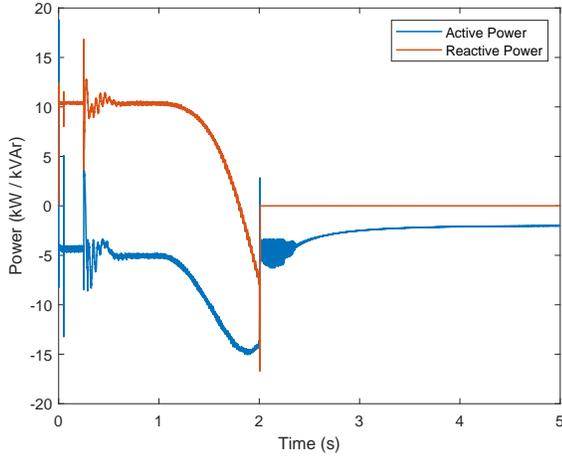
Fig. 5. Active and reactive power exchanged by the microgrid inverter.
