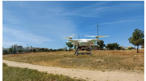
Fig.7. Drone with mounted 5G UE during the field trials
