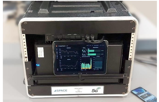
Fig. 2. Satellite edge segment integrated in a portable rack
