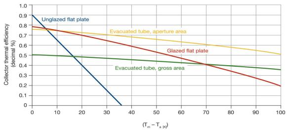
Inlet fluid parameter, °K;  $T_m$  equals mean collector fluid temperature;  $T_a$  equals ambient temperature.
