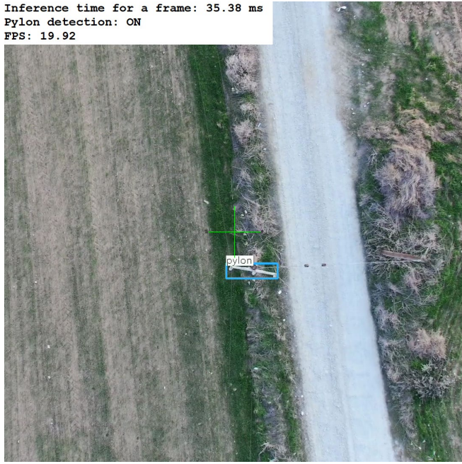
Fig. 3: (a) Pole detection using the tinyYOLOv4 to process, in real-time, video frames on the NVIDIA Jetson Xavier NX embedded platform, and (b) Position correction by aligning the image center (green cross) to the center of bounding box (light blue).
