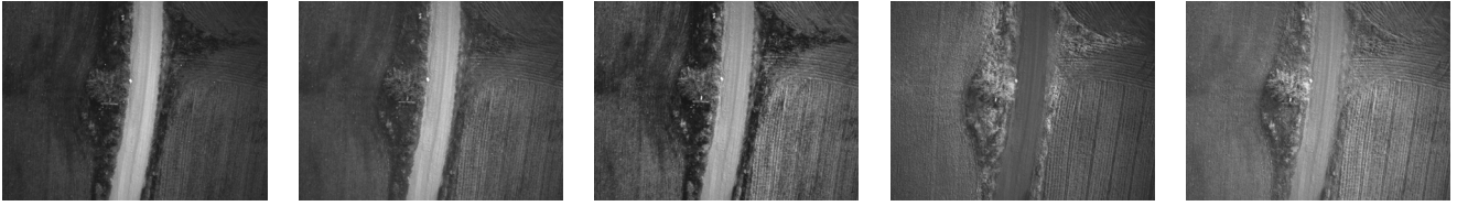
Fig. 5: Multispectral imaging of the power line corridor. From left to right the blue ( 475\pm 32\text{nm} ), green ( 560\pm 27\text{nm} ), red ( 668\pm 14\text{nm} ), red edge ( 717\pm 12\text{nm} ), and near infrared ( 842\pm 57 ) channels are shown [35].
