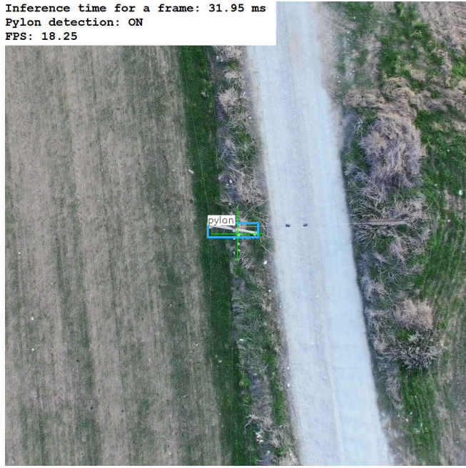
Fig. 3: (a) Pole detection using the tinyYOLOv4 to process, in real-time, video frames on the NVIDIA Jetson Xavier NX embedded platform, and (b) Position correction by aligning the image center (green cross) to the center of bounding box (light blue).
