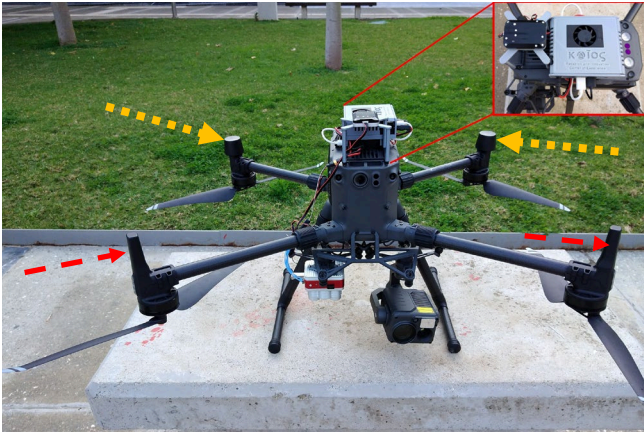
Fig. 1: Equipment for implementing ICARUS inspection platform, consisting of the DJI Matrice 300 RTK UAV, the multi-sensor (RGB and thermal) DJI Zenmuse H20T camera (right downward gimbal), the MicaSense Altum multispectral camera (left downward gimbal) and the NVIDIA Jetson Xavier NX embedded platform (top of UAV; figure inset). Orange dotted and red dashed arrows indicate the differential RTK and transmission antennas, respectively.
