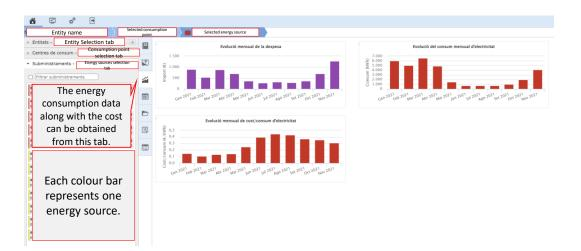
Once a consumption centre has been selected the information regarding its overall energy consumption can be observed and analysed. The specific total consumption by energy source can be selected leading to the information shown above.
