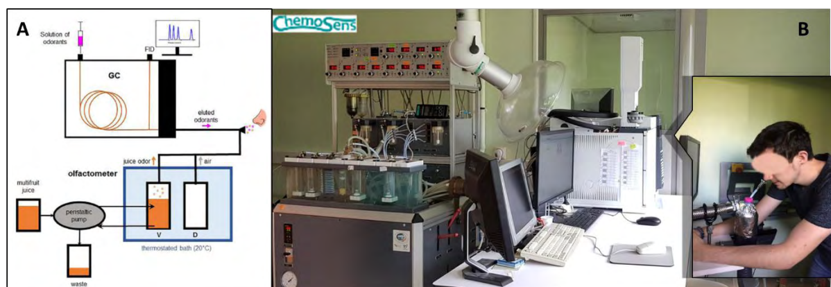
Figure 3: A: Schematic representation of the Olfactoscan device (adapted from Barba et al., 2018 [19]); B: Picture of the experimental setup at the ChemoSens platform of CSGA.
