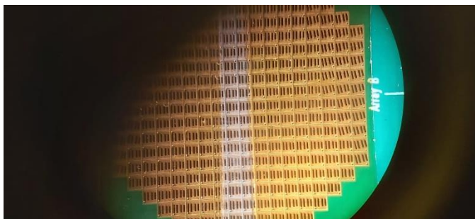
Figure 53: Detail of the LC-RA showing the pixels made of an array of four dipoles.
