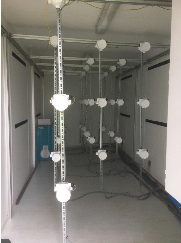
Figure 8 Matrix of sensors on the inside of the container
