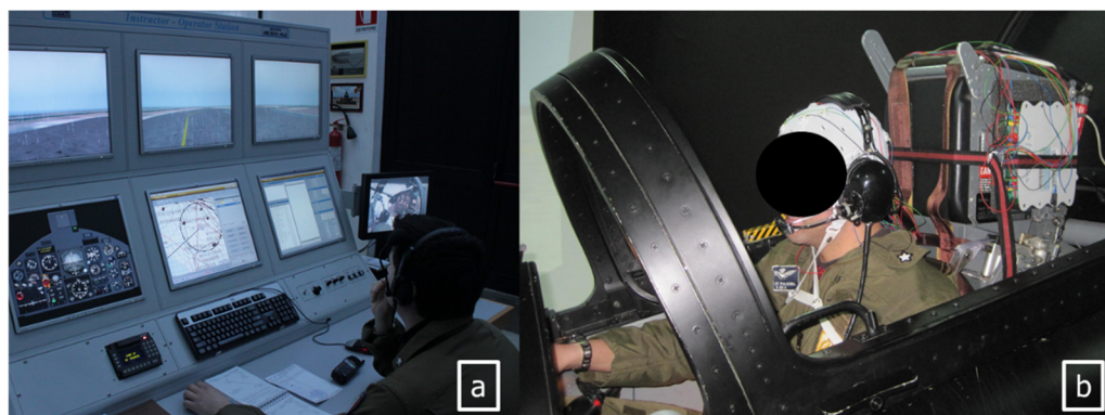
Figure 1. Flight simulator facility at the 61° Stormo in Galatina (Italy): (a) the MB339 alpha simulator platform allowed the instructors to monitor and communicate with the pilots and to interact with the aircraft for inducing three unusual attitudes; (b) the pilots' brain (EEG) and heart (ECG) activity was acquired for the entire flight simulation.
