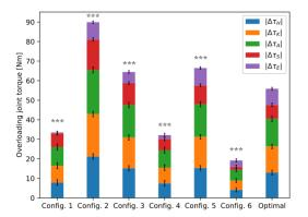
Figure 6: The sum of all overloading joint torques for different configurations<sup>8</sup>. Different colours in the bar represent different contribution from different joints.
