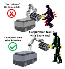
Figure 1: The illustration of the proposed concept. The proposed ergonomic control of human-robot collaboration aims to minimise the effect of overloading joint torques and maximise the arm manipulation ability while performing a repetitive manufacturing task.
