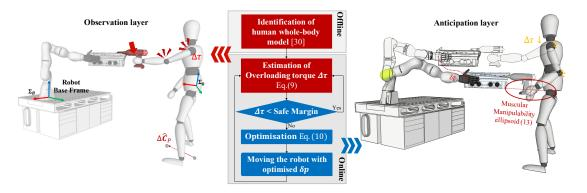
Figure 2: The overall procedure of the proposed method. The observation (left) and the anticipation layer (right) for estimating and reducing the overloading joint torques in human-robot collaboration are illustrated.
