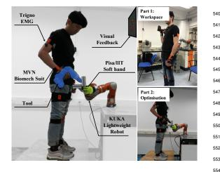
Figure 4: Overview of the experimental setup. The experimental setup consisted of a MVN Biomech suit, a KUKA LBR IV+ equipped with the Pisa/IIT softhand, visual feedback and wireless EMG sensors. The experimental purpose consisted of two parts: task comparison in workspace of the arm, and evaluation in the optimisation.
