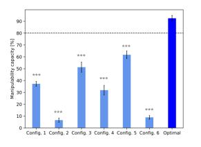
Figure 7: The results<sup>8</sup> of the manipulability capacity for different configurations. The black dashed line denotes the manipulability capacity constraint set in the optimisation process.
