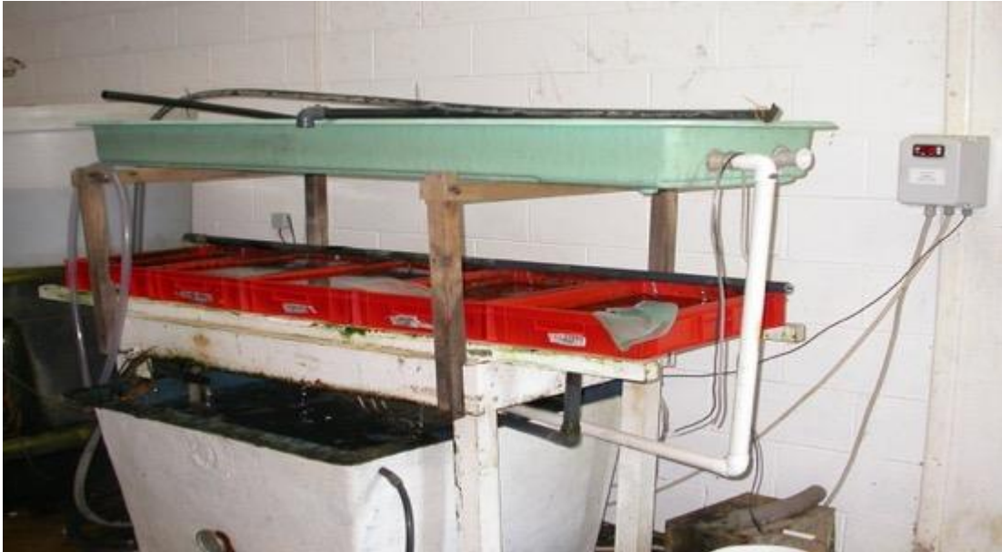
Conditioner showing 5 mussel trays and 1500 l. recirculation reservoir. Photo: I. Connellan
