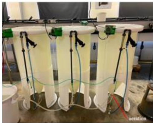
Figure 4. Larval rearing system consisting of 120 L conical tanks and aeration from the bottom. Photos: Clarie Ng
