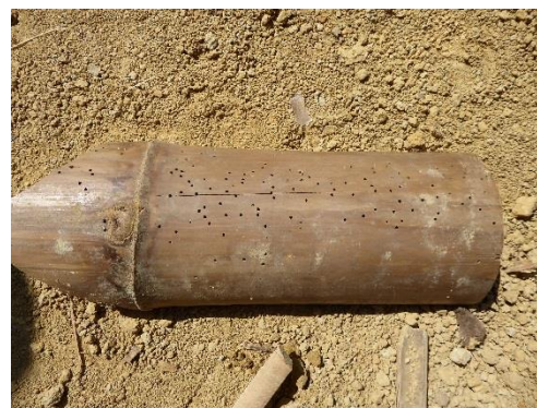
b) Beetle exit holes visible on side of bamboo (Bangladesh) (Kaminski, 2016)
