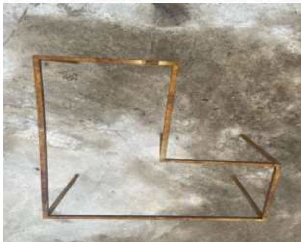
Fig.1:-Basic frame made with mild steel
