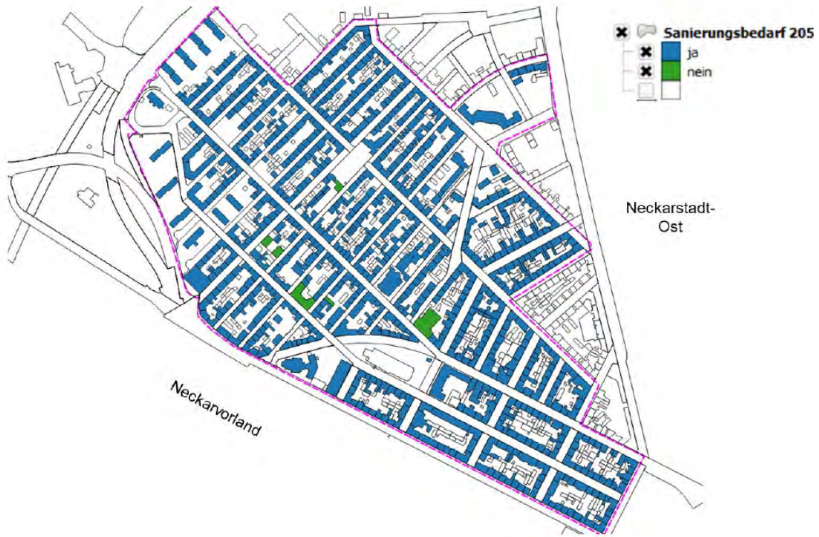
Figure 12: Energetic renovation need of buildings on the ground floor (blue: yes; green: no) (source: MVV Regioplan).
