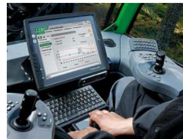
AVATAR, EU/Germany Smart real time feedback and training system for forest machine operators
