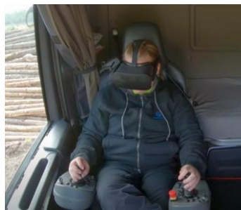
HiVision, Finland Virtual reality support for crane operators
