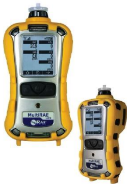
Figure 26. MultiRAE Lite IR natural gas detector
