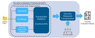
Fig. 4. Overview of the Security Evaluation Framework
