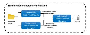
Fig. 7. Overview of the System-wide Vulnerability Prediction
