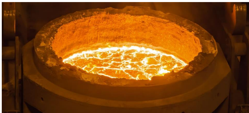
Figure 1: Refractories application (steel ladle) [4]
