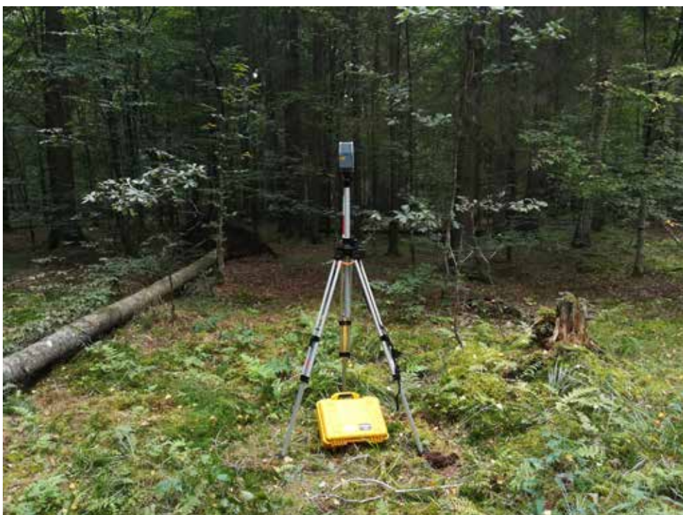
Figure 10.2. Trimble TX5 phase scanner in the process of performing a scan on a sample plot (photo Kamil Pilch)
