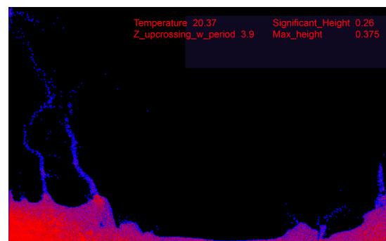
**Figure 3:** Visualisation result. Upper right: Sea wave parameters. Temperature, significant wave height, mean zero crossing wave period, maximum wave height.
