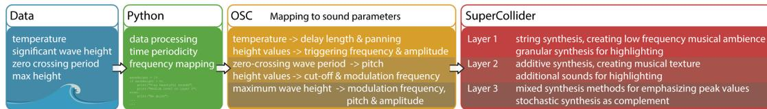
**Figure 2:** The oceanographic data were processed in Python and transmitted via OSC to SuperCollider where various sound parameters were mapped to the data values.
