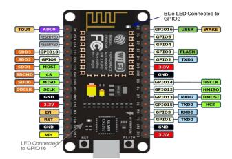
Fig. 2 Pin configuration of ESP8266 [10], [11]
