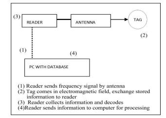
Fig.1 Block diagram showing working of RFID [8]
