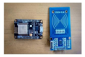
Fig. 3 Photograph of ES8266 and RFID Scanner used
