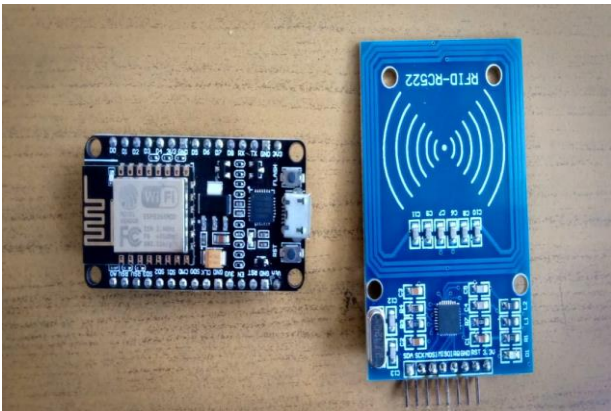
Fig. 3 Photograph of ES8266 and RFID Scanner used
