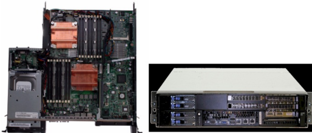
Figure 19 IBM iDataplex dx360M3 server board and 2U chassis with two GPUs.
