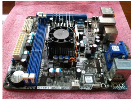
Figure 25 The AMD Brazos E-350 motherboard.
