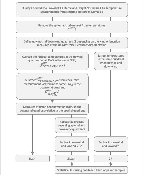
Figure 2. Flowchart diagram showing the different steps undertaken to calculate the downwind urban heat advection (UHA), the upwind-downwind gain/loss heat anomaly  $\Delta$ UHA and the upwind-downwind temperature anomaly  $\Delta$ T.
