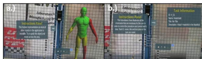
Fig. 4. Training mode introducing a) ergonomic analysis results and b) assembly instruction panels
